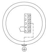
Terminal 3 is internal connected to ground. It is recommended to use a shielded cable for stable measurement.
