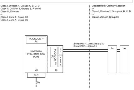
Intrinsically safe parameter of supply and signal circuit
