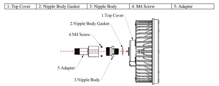
The Top Cover is equipped with the entry hole by mounting the Nipple Assembly.
