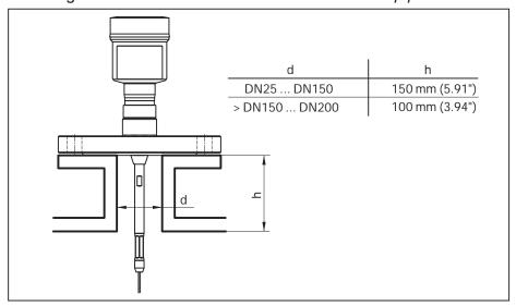
Fig. 4: Mounting socket
