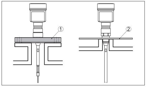
Fig. 3: Mounting in non-metallic vessel
