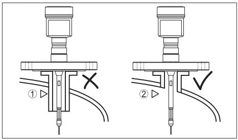
Fig. 5: Socket must be installed flush
