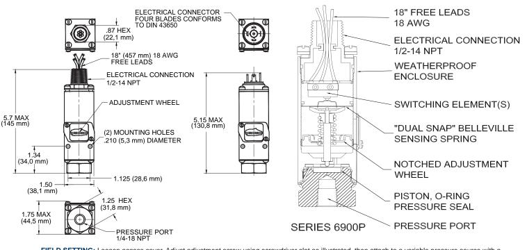
FIELD SETTING: Loosen access cover. Adjust adjustment screw using screwdriver slot as illustrated, then attach to a variable pressure source with a suitable gage, and check that the circuit continuity operates at the pressures desired. Clockwise to increase settings. Counterclockwise to decrease setting.
