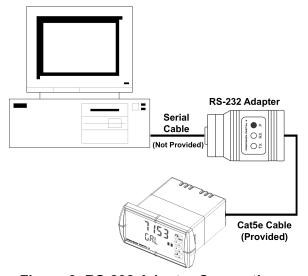
Figure 3. RS-232 Adapter Connections
