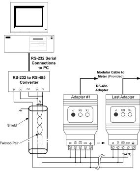
Figure 15. RS-485 Two-Wire Multi-Drop Wiring
