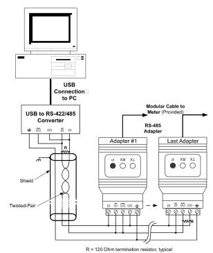
Figure 28. RS-485 Two-Wire Multi-Drop Wiring
