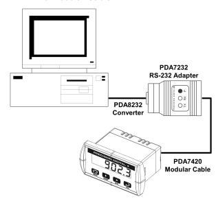
Figure 23. Connections for PDA8232 to serial device
