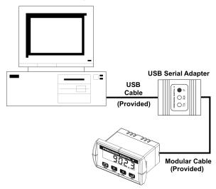
Figure 18. USB Adapter Connections
