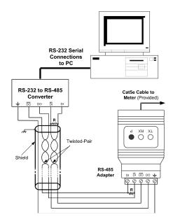
Figure 4. RS-422 or RS-485 Wiring Notes:
