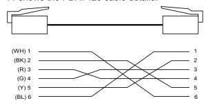
Figure 11. Standard Modular Cable Wiring
