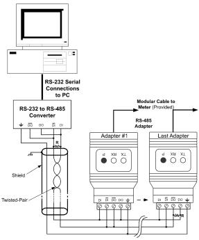
Figure 10. RS-485 Two-Wire Multi-Drop Wiring
