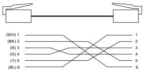
Figure 8. Standard Modular Cable Wiring
