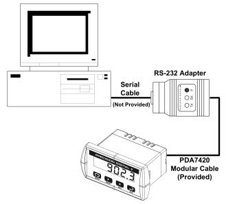
Figure 7. RS-232 Adapter Connections
