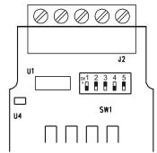
Figure 24. PDA8485 DIP Switch Location
