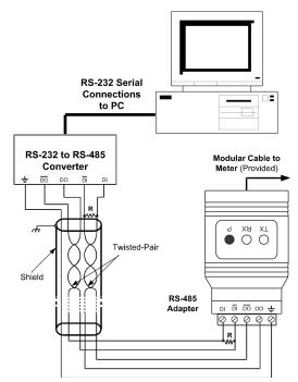
Figure 9. RS-422 or RS-485 Wiring Notes:
