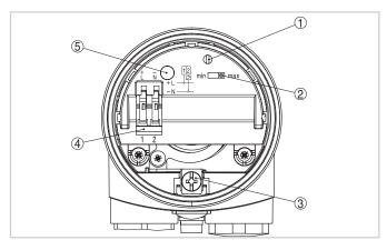
Electronics and connection compartment - contactless electronic switch
