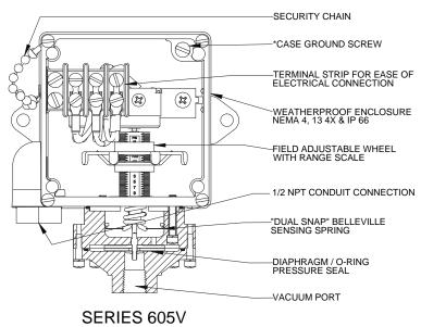
**FIELD SETTING:** Open access cover. Adjust wheel as illustrated. Clockwise to increase settings. Counterclockwise to decrease settings.
