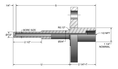
("U" length for non-lagging wells) = "S" - 2" ("U" length for lagging wells) = "S" - 2" - "T" (To solve for "T"), "T" = "S" - "U" - 2" (When "U" and "S" are specified)
