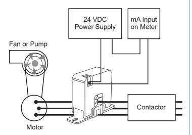
Figure 1: Measuring Current Using PDA6420 Current Transducer
