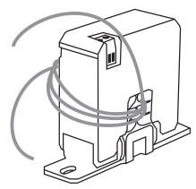
Figure 2: PDA6420 Current Transducer Shown with Four Turns
