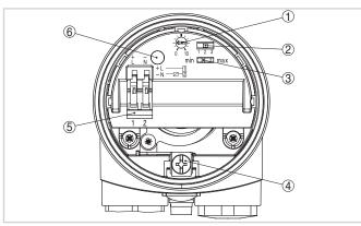
Oscillator - Contactless electronic switch
