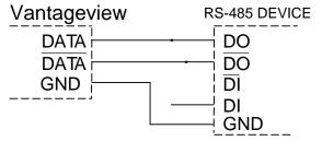
Figure 12. RS-485 4 Wire Serial Connections
