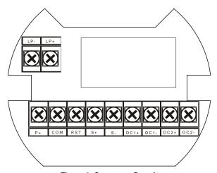
Figure 1. Connector Board
