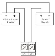
Figure 10. 4-20 mA Output Connections
