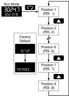
To add a menu or parameter to the menu structure, or change the default menus, press **Enter** at the desired menu in the position (P05) to be edited, and use the **Up** or **Right** arrows to select the desired menu item for that position. See page 33 for a complete list of the available menu selections for each position.
