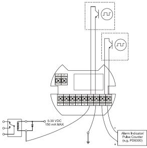
**Figure 13. Open Collector Output Connections**
