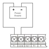
Figure 8. DC Power Connections
