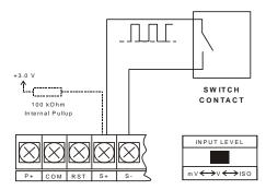
Figure 7. Switch Contact Input (Reed)
