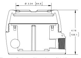
Figure 17. Enclosure Dimensions - Side View
