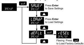
The save feature (**SRUEP**) saves all current parameter settings into the memory of the backup restore. The backup restore feature is loaded with factory default settings until a new configuration is saved.
