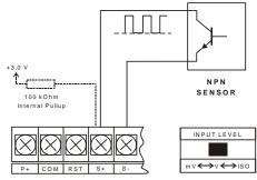
Figure 5. NPN Open Collector Input (NPN)
