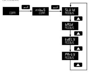
Modbus communications is performed with the 2-wire RS-485 with Modbus RTU option.
