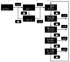
Output 1 and 2 Setup (OUT 1, OUT 2)
