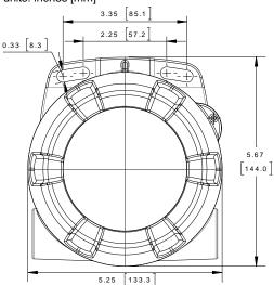
Figure 16. Enclosure Dimensions - Front View
