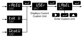
Fully alphanumeric values are set using the **Right** button to select the digit to be changed. Press the **Up** button to begin editing the digit, then the **Up** and **Right** arrow buttons to select the next or previous alphanumeric character. Press the **Enter** button to confirm and select the next digit to change.
