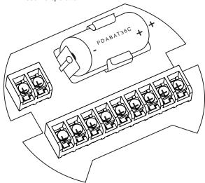
Figure 14. Battery Orientation
