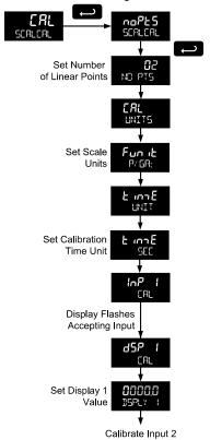
The multi-point linearization feature (naPt5) can be used to linearize the display for non-linear signals. For instructions on how to utilize this feature, see Multi-Point Linearization (naPt5), page 30.
