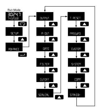
Advanced menus R OUT displayed only for meters with the analog output option, COMM displayed only for meters with the serial communications option, and STRNDBY only for meters with battery or battery backup power.
