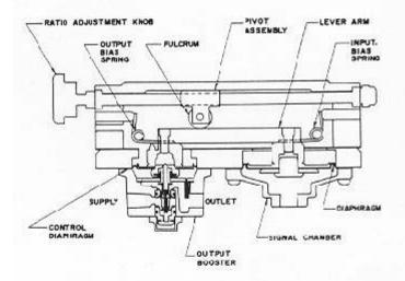
Output pressure is a function of signal pressure times the ratio of lever arm lengths on either side of the fulcrum.
