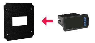
2 Take the mounting plate with the meter and screw it onto the enclosure box by lining up the four screw holes on the plate to the four mounting rods shown on the inside the of enclosure.
