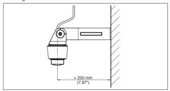
Fig. 4: Mounting via a mounting bracket
