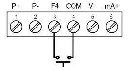
Figure 16: F4 Digital Input Connections
