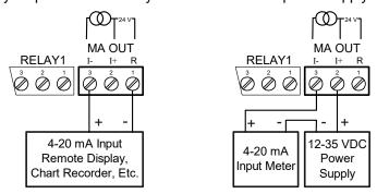
Figure 17: 4-20 mA Output Connections
