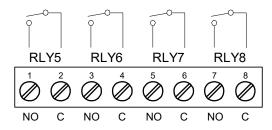
Figure 19: External Relays Module Connections
