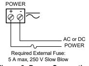
**Figure 6: Power Connections**
