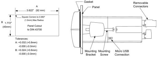
Figure 1: 1/8 DIN Panel Mounting
