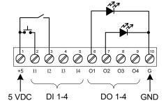
Figure 20: Digital I/O Module Connections
