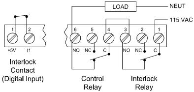
**Figure 21: Interlock Connection**
