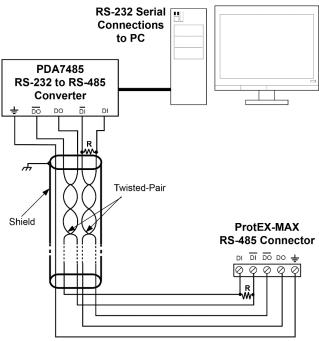
Figure 10: RS-485 Wiring
