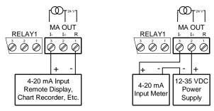
Figure 16. 4-20 mA Output Connections
