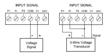
Figure 7. Voltage Input Connections
