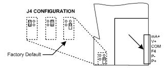
Figure 1. Transmitter Supply Voltage Selection
