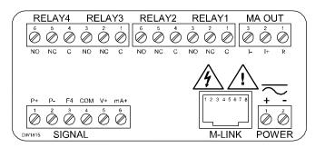
Figure 3. Connector Labeling for Fully Loaded PD6001
