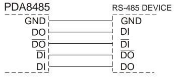
Figure 20: General Four-Wire Network Connection
