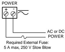
**Figure 4. Power Connections**
