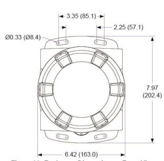
Figure 22: Enclosure Dimensions - Front View
