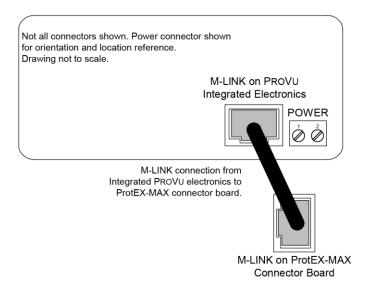
Figure 2: Integrated ProVu Required Connections
