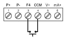
Figure 15. F4 Digital Input Connections
