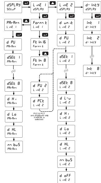
After setting up the input and display, press the Menu button to exit programming and skip the rest of the setup menu. Press the Menu button again and the Up arrow to reach the *Program* menu and complete the scaling or calibration of the meter.
