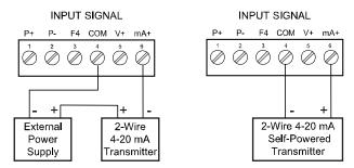
Figure 6. Transmitter Powered by Ext. Supply or Self-Powered
