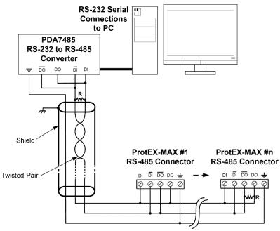
Figure 11: RS-485 Two-Wire Multi-Drop Wiring
