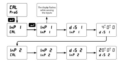
Warm up the meter for at least 15 minutes before performing calibration to ensure specified accuracy.
