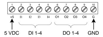
Figure 18: Digital I/O Connections
