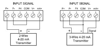
Figure 5. Transmitters Powered by Internal Supply
