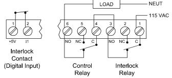
Figure 17. Interlock Connections
