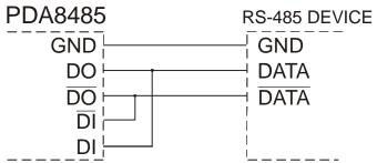
Figure 21: General Two-Wire Network Connection
