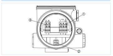
Connection compartment double chamber housing
