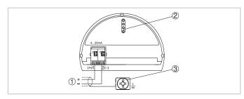
Electronics and connection compartment, single chamber housing
