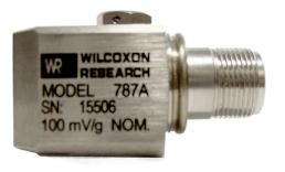
Wilcoxon's side-exit 100 mV/g broadband sensor is ideal for monitoring machine vibration on a wide range of rotating equipment including motors, pumps, fans, compressors, turbines and generators. A 316L stainless steel casing provides rugged durability for the most extreme environments. The sensing element is housed in a case-isolated Faraday shield, providing maximum protection from ground loops and RF interference.
