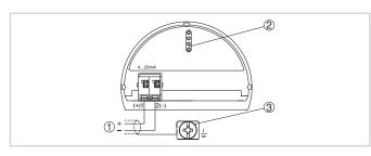
Electronics and terminal compartment, single chamber housing
