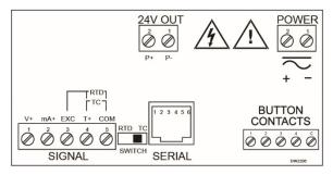
Figure 14. Connector Labeling for PD765-6X0-10
