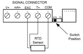
Figure 27. Three-Wire RTD Input Connections
