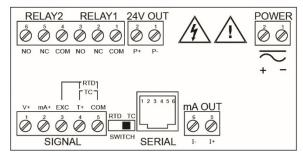
Figure 12. Connector Labeling for PD765-6R5-10
