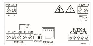
Figure 17. Connector Labeling for PD765-#X3-00
