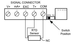
Figure 29. Four-Wire RTD Input Connections
