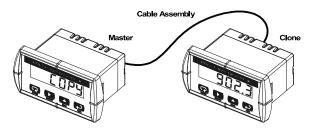
Figure 39. Meter Copy Connection
