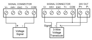
Figure 25. Voltage Input Connections
