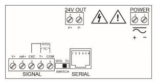
Figure 5. Connector Labeling for PD765-6R0-10
