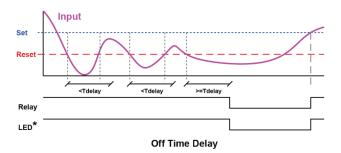
If the signal crosses the set point, the On time delay timer starts and the relay trips when the time delay has elapsed. If the signal drops below the set point (high alarm) before the time delay has elapsed, the On time delay timer resets and the relay does not change state. The same principle applies to the Off time delay.
