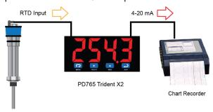
Connections for the 4-20 mA transmitter output are made to the connector terminals labeled "mA OUT: I-, I+". The 4-20 mA output may be powered from an internal power supply (optional) or from an external power supply.
