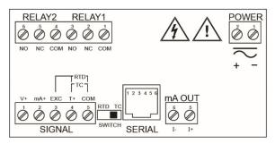
Figure 11. Connector Labeling for PD765-7R5-00
