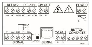
Figure 21. Connector Labeling for PD765-6X5-10
