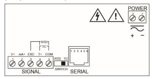
Figure 4. Connector Labeling for PD765-#R0-00
