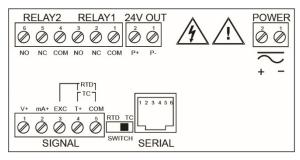
Figure 7. Connector Labeling for PD765-6R2-10
