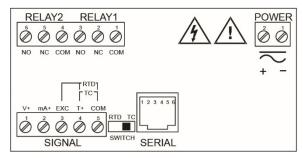
Figure 6. Connector Labeling for PD765-#R2-00
