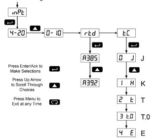
If RTD is selected, the display shows **R3B5** or **R392**. Select the coefficient to match the RTD sensor, either 0.00385 (**R3B5**, European curve) or 0.00392 (**R392**, American curve). The display then shows the decimal point menu, **dEc.P**. Select the decimal point resolution as shown on page 22.
