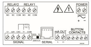
Figure 20. Connector Labeling for PD765-7X5-00
