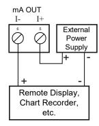
Figure 35. 4-20 mA Output Powered Externally
