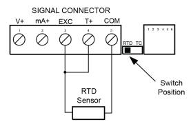
Figure 28. Two-Wire RTD Input Connections
