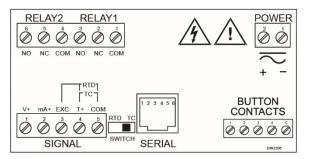
Figure 15. Connector Labeling for PD765-#X2-00
