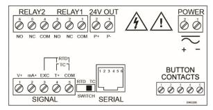
Figure 16. Connector Labeling for PD765-6X2-10
