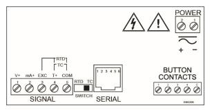
Figure 13. Connector Labeling for PD765-#X0-00
