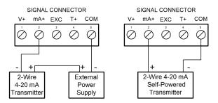
Figure 24. Transmitter Powered by External Supply or Self-Powered
