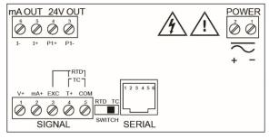
Figure 9. Connector Labeling for PD765-6R3-10
