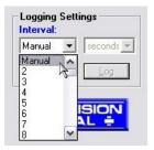
Logging may be paused or stopped at any time. MeterView will indicate logging and paused status with corresponding message flashing in the main window status bar. When logging, all other MeterView functions and windows are not accessible.
