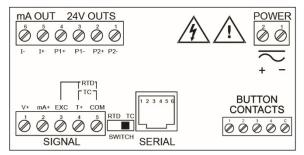
Figure 19. Connector Labeling for PD765-6X3-20
