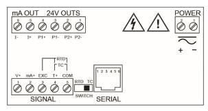
Figure 10. Connector Labeling for PD765-6R3-20
