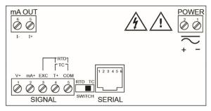
Figure 8. Connector Labeling for PD765-#R3-00
