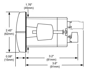
Figure 2. Meter Dimensions - Side View
