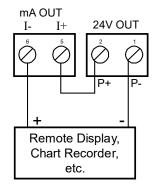
Figure 34. 4-20 mA Output Powered by Meter
