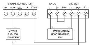
Figure 33. 4-20 mA Output & Input Signal Powered by Meter
