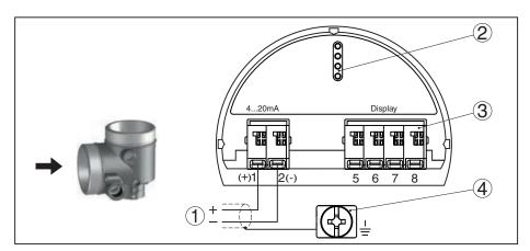
Fig. 5: Connection compartment - double chamber housing
