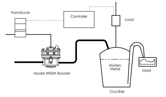
Figure 2. Automated Crucible Despencing
