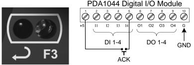
Figure 22: Acknowledge Relays w/Function Key or Digital Input Setting Up the Interlock Relay (Force On) Feature
