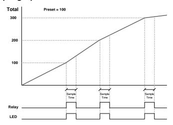
When the total reaches the preset, the relay trips and the sample time starts. After the sample time has elapsed, the relay resets. The cycle repeats every time the preset value is added to the total.
