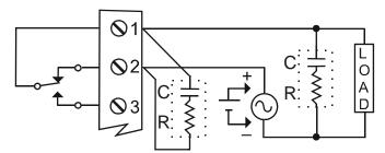
Figure 16: AC and DC Loads Protection
