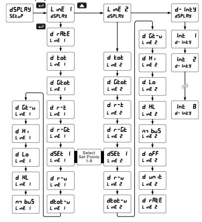
Display Intensity: The meter has eight display intensity levels to give the best performance under various lighting conditions. Select intensity 8 for outdoor applications. The default display intensity setting is 8.
