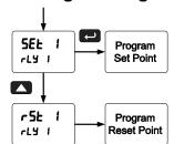
High alarm indication: program set point above reset point. Low alarm indication: program set point below reset point. The deadband is determined by the difference between set and reset points. Minimum deadband is one display count. If the set and reset points are programmed with the same value, the relay will reset one count below the set point. Note: Changes are not saved until the reset point has been
