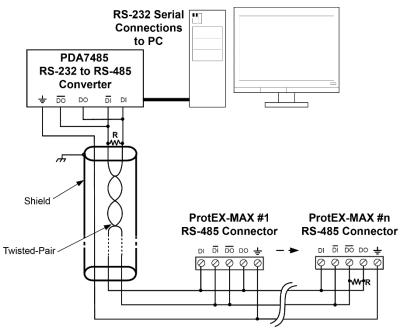
Figure 14: RS-485 Two-Wire Multi-Drop Wiring
