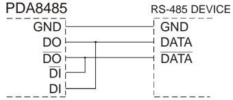
Figure 24: General Two-Wire Network Connection
