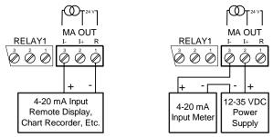
Figure 19: 4-20 mA Output Connections
