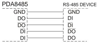
Figure 23: General Four-Wire Network Connection
