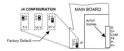
Figure 1: Transmitter Supply Voltage Selection
