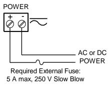
**Figure 4: Power Connections**
