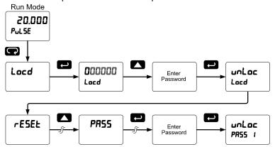
If the correct six-digit password is entered, the meter displays the message unlocked) and the protection is disabled until a new password is programmed.
