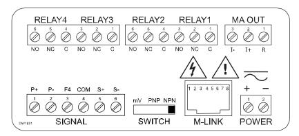
Figure 3: Connector Labeling for Fully Loaded PD6300
