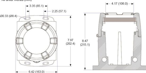
Figure 25: Enclosure Dimensions – Front View
