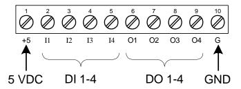
Figure 21: Digital I/O Connections
