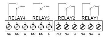
Figure 15: Relay Connections
