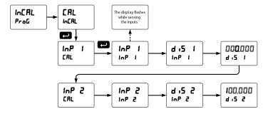
**Note:** The display values (d · 5 · 1 and d · 5 · 2) need to be in units of measure per second.
