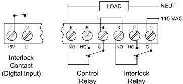
**Figure 20: Interlock Connections**
