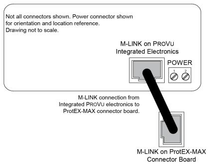
Figure 2: Integrated ProVu Required Connections
