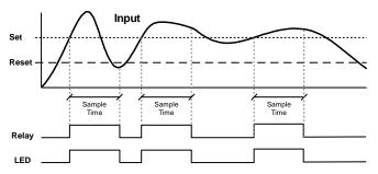
When the signal crosses the set point, the relay trips and the sample time starts. After the sample time has elapsed, the relay resets. The cycle repeats every time the set point is crossed, going up for high alarms and going down for low alarms.
