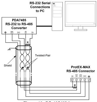
Figure 13: RS-485 Wiring
