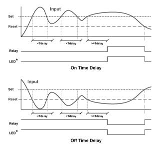
When the signal crosses the set point, the *On* time delay timer starts and the relay trips when the time delay has elapsed. If the signal drops below the set point (high alarm) before the time delay has elapsed, the *On* time delay timer resets and the relay does not change state. The same principle applies to the *Off* time delay.
