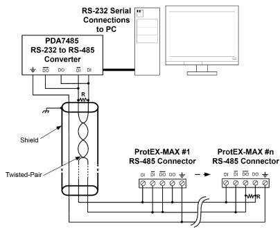
Figure 11: RS-485 Two-Wire Multi-Drop Wiring
