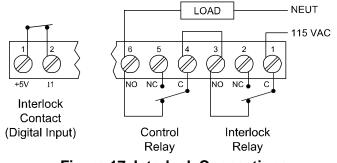
Figure 17. Interlock Connections
