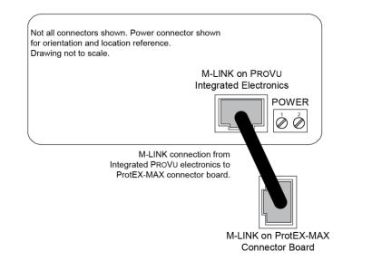
Figure 2: Integrated ProVu Required Connections
