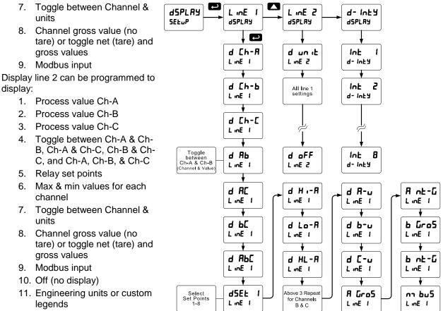
**Display Intensity:** The meter has eight display intensity levels to give the best performance under various lighting conditions. Select intensity 8 for outdoor applications. The default intensity setting is 8.
