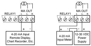
Figure 16. 4-20 mA Output Connections
