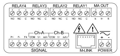
Figure 3. Connector Labeling for Fully Loaded PD6060
