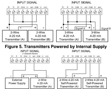
Figure 6. Transmitter Powered by Ext. Supply or Self-Powered
