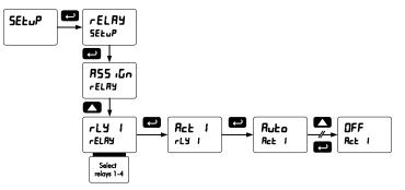
2. In the Advanced features – User menu program any of the digital inputs to Force On any of the internal relays (1-4).
