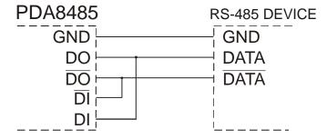
Figure 21: General Two-Wire Network Connection
