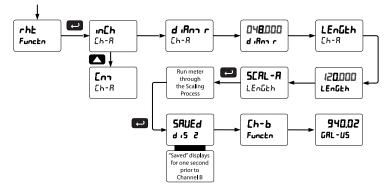
Note: After Scale is displayed continue pressing the Enter button until the meter completes the scaling of the input and display values.
