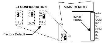
Figure 1. Transmitter Supply Voltage Selection
