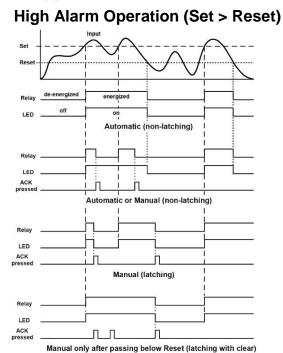
For Manual reset mode, ACK can be pressed anytime to turn "off" relay. To detect a new alarm condition, the signal must go below the set point, and then go above it.
