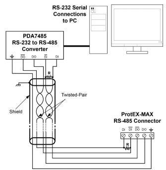
Figure 10: RS-485 Wiring
