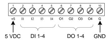
Figure 18: Digital I/O Connections
