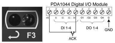
Figure 19. Acknowledge Relays w/Function Key or Digital Input
