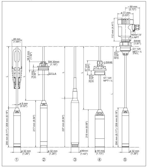
Fig. 18: VEGAWELL 52, with transmitter Duplex steel (1.4462)/PVDF
