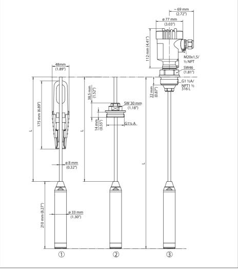
Fig. 17: VEGAWELL 52, with transmitter 316L/Titanium 33 mm
