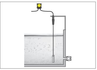
Fig. 5: Mounting example: VEGAWELL 52 in an open basin with breather housing VEGABOX 03
