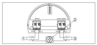
Fig. 13: Wiring plan VEGAWELL 52 for 4 ... 20 mA sensors
