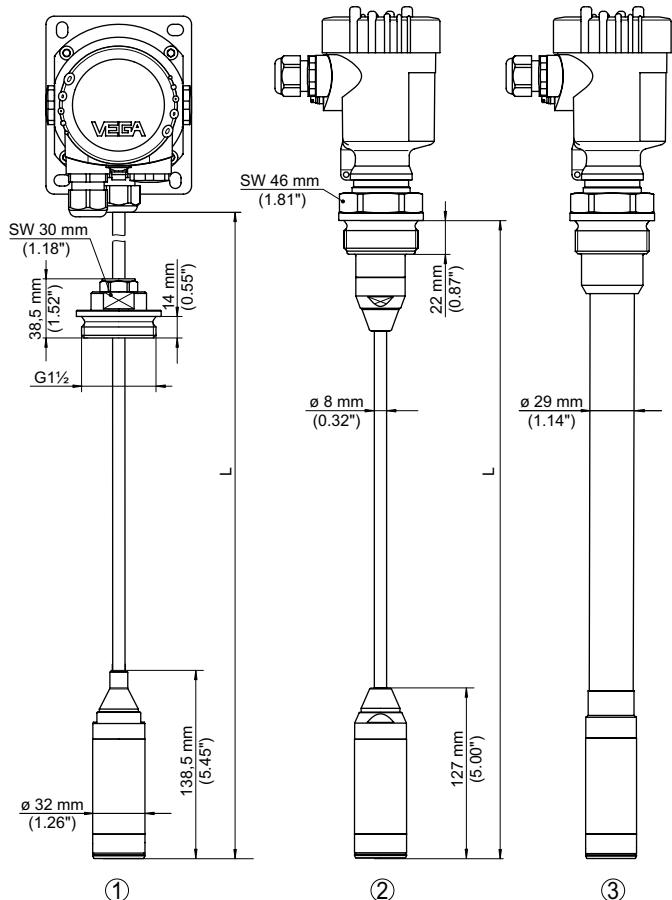
① Version with suspension cable, threaded fitting unassembled G1½ and cable outlet / IP 68, external housing plastic / IP 65
