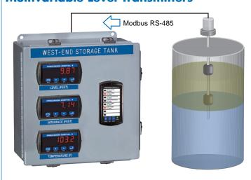
The top Snooper is displaying product level and it is set up as a master device to the level transmitter's slave device. The next two Snoopers are set up in Snooper mode and they are displaying interface and product temperature. Each Snooper's two relays are connected to the PD158 annunciator to indicate alarm conditions.
