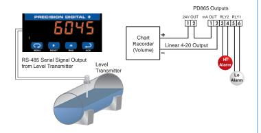
The Snooper's multi-point linearization feature can be used to display the volume in a round horizontal tank or any other non-linear vessel. In addition, it can generate a 4-20 mA output that is linear to volume.
