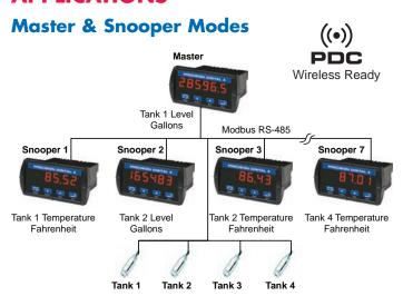
In this application, the PD865 at the top is acting as the Master and requests eight process variables (level & temperature) by polling four multivariable tank level sensors. Seven of these variables are polled by the master on behalf of the seven PD865s acting in Snooper mode (a process called proxy polling). The seven PD865s display specific data captured during the polling process without detection by, or interfering with, either the master or slaves on the network.
