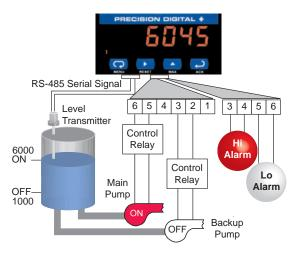
The Snooper, in conjunction with a Modbus output level transmitter, can be used to control and alternate up to four pumps. In the application above, the Snooper's two Form C relays are being used to control and alternate the Main and Backup pumps, and the Snooper's two Form A relays are being used for High and Low Alarm.
