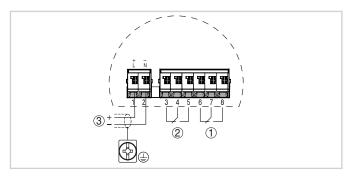
Wiring plan, Receiving unit - VEGAMIP R62 R (receiver)
