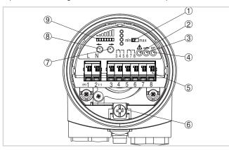
Electronics module receiving unit MP60EE.R - Relay output
