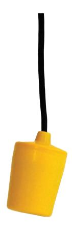
Series TLS Cable Float Switches are dual-point switches that provide built-in hysteresis for better pump control. The switch operating levels are easily adjustable based on the cable weight location, and the floats are especially suited for use in waste water and sewage applications with low specific gravity.
