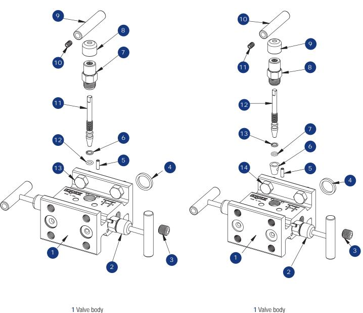
2 Blue dust cap 3 Plug 4 Gasket ring 5 Slotted spring pin 6 PTFE back-up ring 7 Valve bonnet 8 Green dust cap 9 Valve "T" handle 10 Set screw 11 Valve stem
