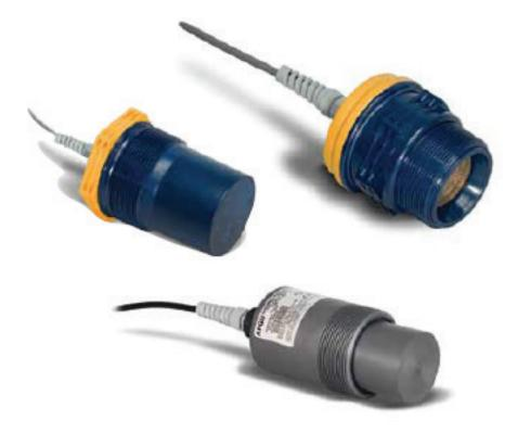
The DST series ultrasonic sensors are designed to be used in conjunction with a DCR controller to give you a simplified, stand-alone system. The transmit and receive circuit is built into the sensor and digitally communicates the detected distance to the DCR controller. This allows the sensor to be separated from the DCR controller by up to 2000 feet with no signal loss. With several sensors to choose from, there are plenty of options for your application needs.
