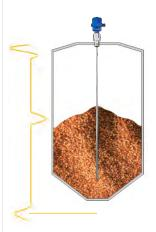
When the silo is filled with material, the negative downturn in the echo curve appears further away due to the lower propagation speed of the microwave pulse in the material. For the echo processing software, the probe appears to be longer than it actually is
