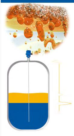
TDR sensors process the echo signals in envelopes. The width and slope of the envelope is largely determined by the bandwidth. The larger the bandwidth, the steeper and narrower the envelope. A higher bandwidth consequently leads to a better resolution, as a result of which two echo signals in quick succession can be better separated from one another. Steeper envelopes also increase accuracy.
