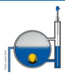
To measure the water level in steam boilers, TDR sensors are installed in a bypass pipe. Steam compensation helps to precisely determine the fill level even at an operating pressure of over 40 bar and a temperature of over 200°C
