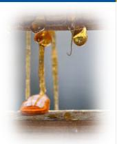
Cement or flour are classic examples of the fact that build-up can sometimes occur on parts in contact with the process in solid applications. With TDR sensors, such a process-contacting part is the probe. It is either a rod or a rope. The respective surfaces are designed in such a way that **product deposits are minimized**. In addition, the rope variants can be covered with a **PA coating**.
