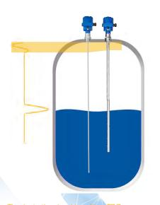
Thanks to the signal bundling, TDR sensors with a coaxial probe can still detect signals in close range. This enables the tank to be filled up to the top edge.
