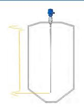
If the silo is empty, the negative downturn in the echo curve and the actual end of the probe match
