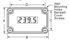
Figure 4. Case Dimensions – Front View
