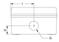
Figure 6. Case Dimensions – Bottom View
