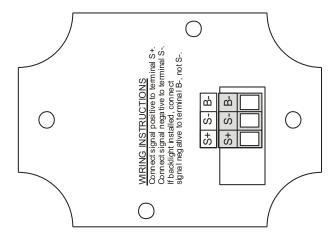
Figure 1. PD662 Mounting Board Rear View
