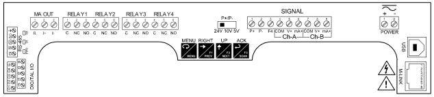
Figure 7. Connector Labeling for Fully Loaded PD2-6080/1
