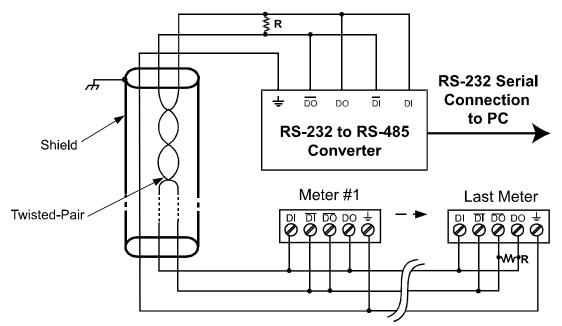
Figure 11. RS-485 Two-Wire Multi-Drop Wiring
