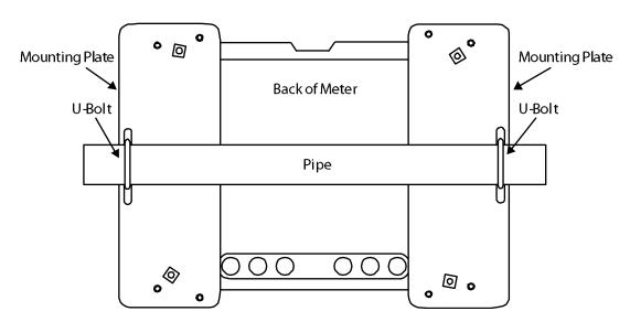
Figure 5. Horizontal Pipe Mount Assembly
