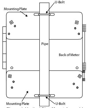
Figure 4. Vertical Pipe Mount Assembly
