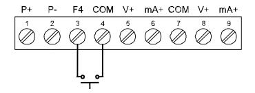
Figure 15. F4 Digital Input Connections
