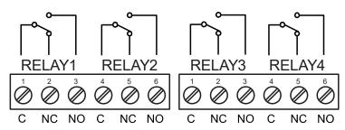
Figure 16. Relay Connections
