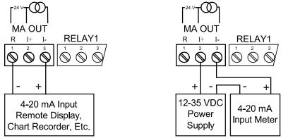
Figure 19. 4-20 mA Output Connections
