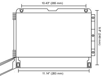
Figure 1. Meter Mounting Holes
