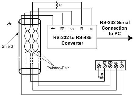
Figure 10. RS-422 or RS-485 Wiring
