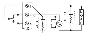
Figure 17. AC and DC Loads Protection
