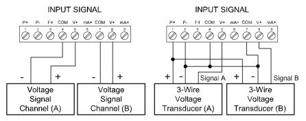
Figure 23. Voltage Input Connections
