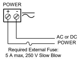
**Figure 8. Power Connections**
