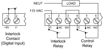
Figure 20. Interlock Connections
