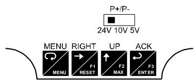
Figure 6. Transmitter Supply Voltage Selection
