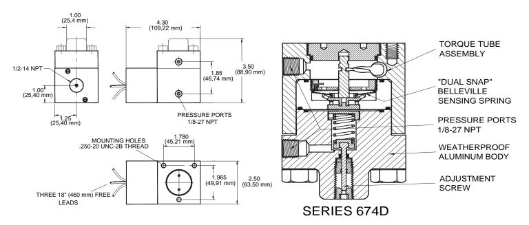
FIELD SETTING: Loosen access cover. Adjust screwdriver adjustment slot. Clockwise to decrease settings. Counterclockwise to increase settings.
