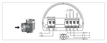
Connection compartment with double chamber housing - low voltage You can find details on electrical connection in the instrument operating instructions at <a href="https://www.vega.com/downloads">www.vega.com/downloads</a>.
