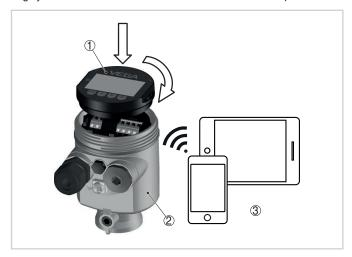
Wireless connection of the sensor to smartphones/tables via Bluetooth
