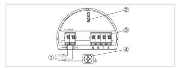
Electronics and terminal compartment, single chamber housing
