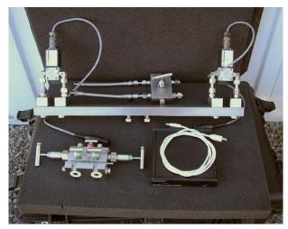
Figure 2: SRE6 and GLE6 test equipment that enables operator to perform an SRE and GLE test simultaneously.
