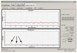
**Figure 1:** A graph exhibits three separate pulsation peaks. The operator can isolate the pulsation source by using new software filtering capability and modifying conditions in the new field. Minimizing and eliminating the pulsation source can ultimately improve the meter's measurement accuracy.
