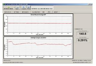
Figure 6: A noise test that would result in  $\Delta P$  difference of 0.291%
