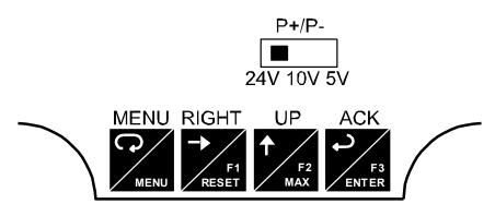
Figure 6. Transmitter Supply Voltage Selection
