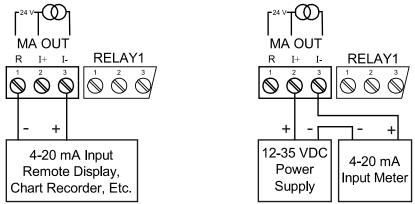
Figure 21. 4-20 mA Output Connections
