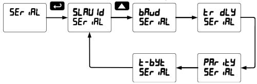
When using more than one meter in a multi-drop mode, each meter must be provided with its own unique address. The meter address (Slave ID) may be programmed between 1 and 247. The transmit delay may be set between 0 and 199 ms. The parity can be set to even, odd, or none with 1 or 2 stop bits.
