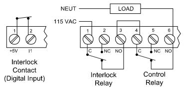
Figure 22. Interlock Connections
