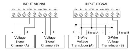
**Figure 11. Voltage Input Connections**
