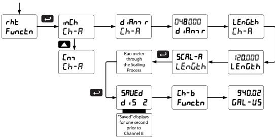
Note: After Scale is displayed continue pressing the Enter button until the meter completes the scaling of the input and display values.
