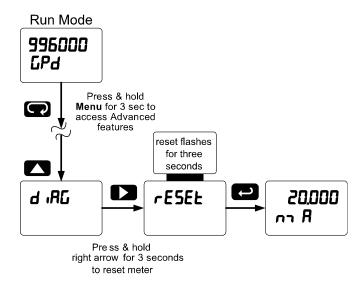
Note: The dual-scale selection for some level applications (d-SCAL) is not reset to the single scale factory default. This can be changed using the Setup – Input menu.
