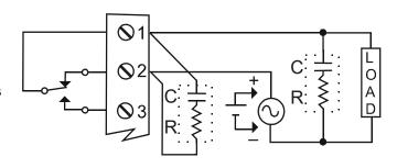
Figure 13. AC and DC Loads Protection
