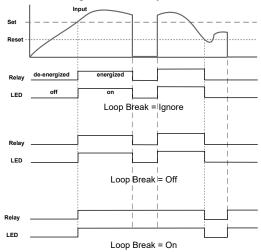
When the meter detects a break in the 4-20 mA loop, the relay will go to one of the following selected actions:
