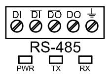
The RS-485 connector has three diagnostic LEDs: a Power (PWR)
