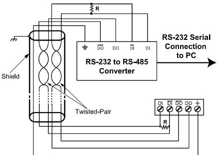
Figure 15. RS-422 or RS-485 Wiring
