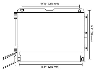
**Figure 1. Meter Mounting Holes**
