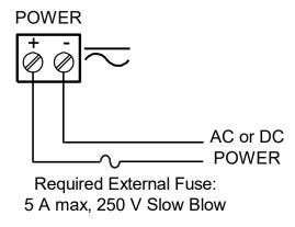
Figure 8. Power Connections
