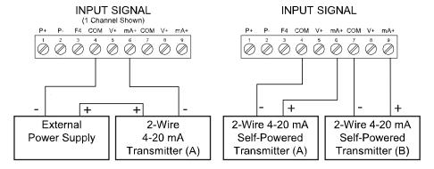
Figure 10. Transmitter Powered by Ext. Supply or Self-Powered
