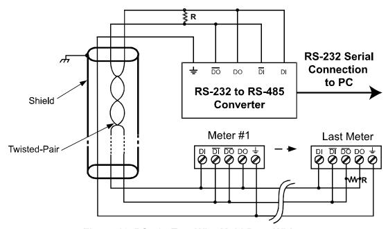
Figure 16. RS-485 Two-Wire Multi-Drop Wiring
