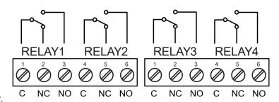
Figure 12. Relay Connections
