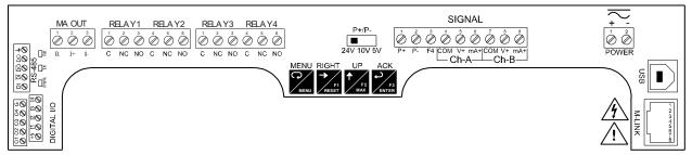
Figure 7. Connector Labeling for Fully Loaded PD2-6060
