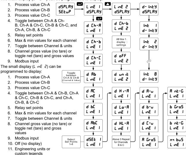
**Display Intensity:** The meter has eight display intensity levels to give the best performance under various lighting conditions. Select intensity 8 for outdoor applications. The default intensity setting is 8.
