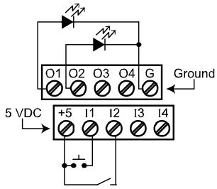
Figure 19. Digital Input and Output Connections
