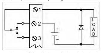
Figure 14. Low Voltage DC Loads Protection
