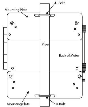
Figure 4. Vertical Pipe Mount Assembly
