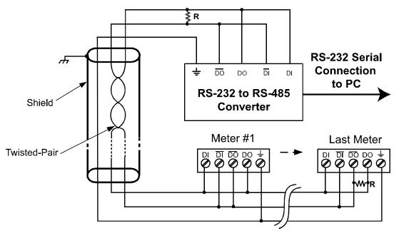
Figure 20. RS-485 Two-Wire Multi-Drop Wiring
