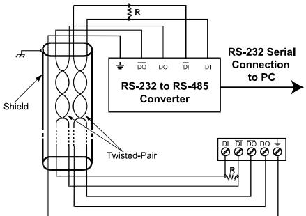
Figure 19. RS-422 or RS-485 Wiring
