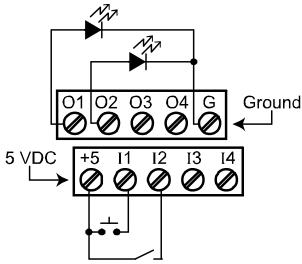
Figure 23. Digital Input and Output Connections
