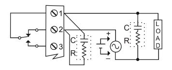
Figure 17. AC and DC Loads Protection
