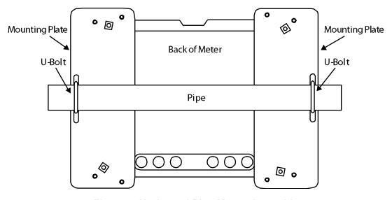
Figure 5. Horizontal Pipe Mount Assembly
