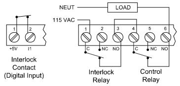
Figure 26. Interlock Connections
