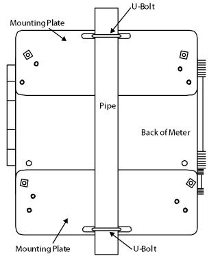
Figure 4. Vertical Pipe Mount Assembly
