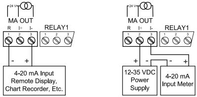
Figure 25. 4-20 mA Output Connections
