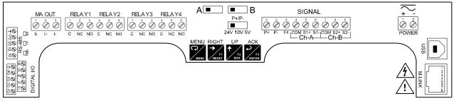
Figure 7. Connector Labeling for Fully Loaded PD2-6363
