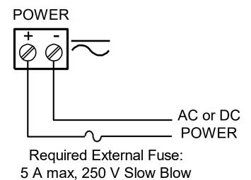
**Figure 8. Power Connections**
