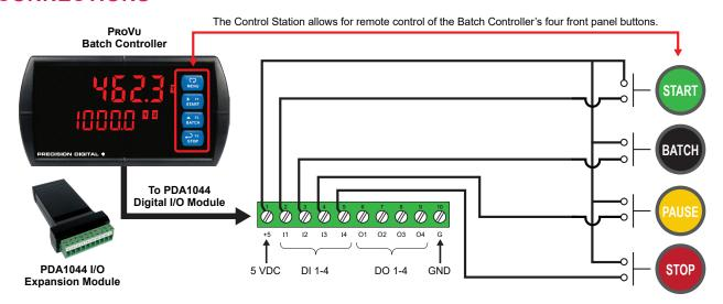
Use the PDA2364-SBPS to remotely operate the ProVu Batch Controller
