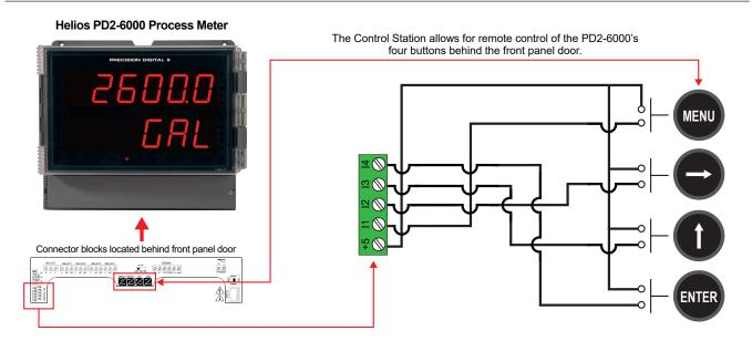
Use the PDA2364-MRUE to remotely control the PD2-6000's four internal programming and operation buttons which are located behind the door below the display.
