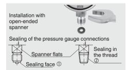
sealing face ①. With tapered threads (e.g. NPT threads), sealing is made in the threads ② using additional sealing materials, e.g. PTFE tape (EN 837-2).
