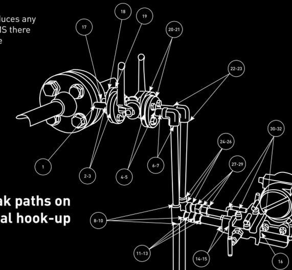
Potential leak paths on a typical hook-up
