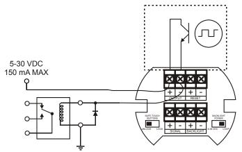
Figure 7. Output Connections
