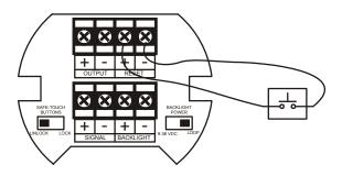
Figure 5. External Alarm Reset/Acknowledge Connections
