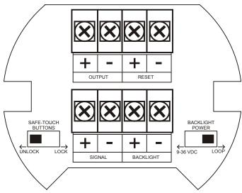
Figure 1. Connector Board
