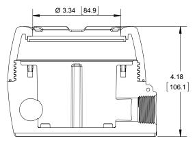
Figure 9. Enclosure Dimensions - Side Cross Section View
