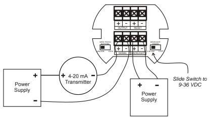
Figure 4. Input Connections with Externally-Powered Backlight
