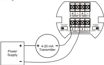
Figure 2. Input Connections without Backlight
