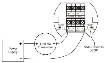
Figure 3. Input Connections with Loop-Powered Backlight
