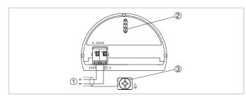
Electronics and terminal compartment, single chamber housing
