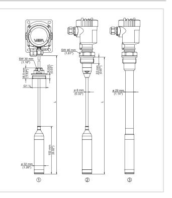
1 Version with suspension cable and threaded fitting unassembled  $G1\frac{1}{2}$
