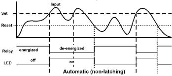
Note: Relay coil is energized in non-alarm condition. In case of power failure, relay will go to alarm state.
