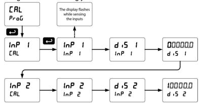
**Note:** The display values (d .5 1 and d .5 2) need to be in units of measure per second.
