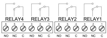
Figure 18: Relay Connections
