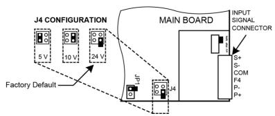
Figure 4: Transmitter Supply Voltage Selection
