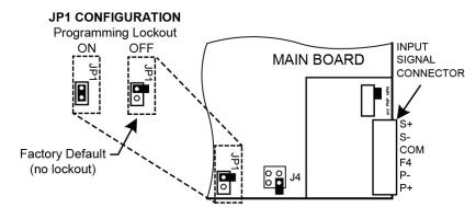
Figure 5: Programming Lockout Jumper Selection
