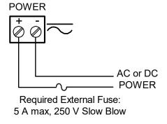
**Figure 11: Power Connections**
