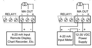
Figure 22: 4-20 mA Output Connections
