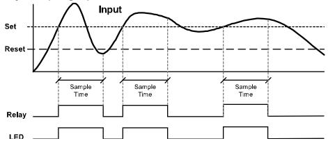
When the signal crosses the set point, the relay trips and the sample time starts. After the sample time has elapsed, the relay resets. The cycle repeats every time the set point is crossed, going up for high alarms and going down for low alarms.
