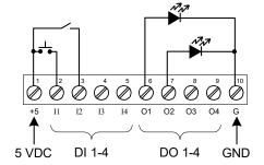
Figure 25: Digital I/O Module Connections
