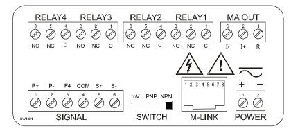
Figure 10: Connector Labeling for Fully Loaded PD6310
