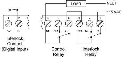
**Figure 26: Interlock Connection**
