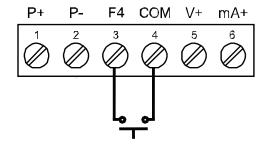
Figure 21: F4 Digital Input Connections
