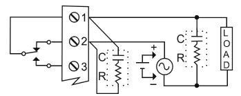
Figure 19: AC and DC Loads Protection
