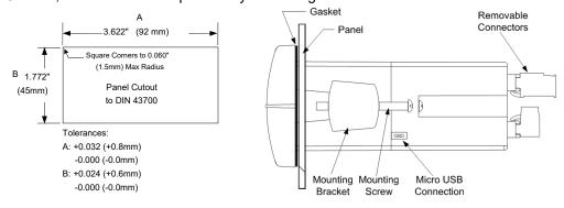
Figure 1: 1/8 DIN Panel Mounting
