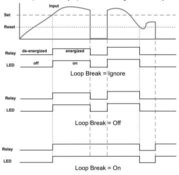
When the meter detects a break in the current or voltage loop, the relay will go to one of the following selected actions:
