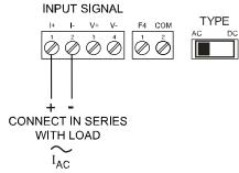
**Figure 9. AC Current Connections**
