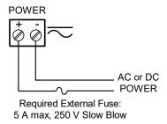
Figure 6. Power Connections
