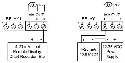
Figure 19. 4-20 mA Output Connections
