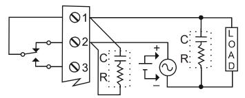
Figure 16. AC and DC Loads Protection
