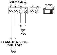
Figure 14. DC Current and Voltage Connections
