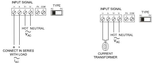
Figure 12. AC Current and Voltage Connections
