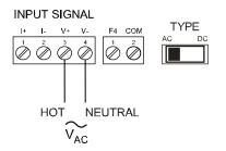
Figure 7. AC Voltage Input Connection
