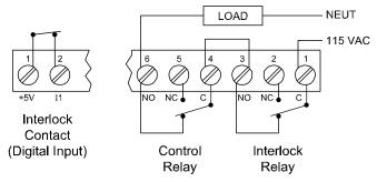
Figure 20. Interlock Connections
