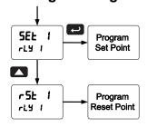
High alarm indication: program set point above reset point. Low alarm indication: program set point below reset point. The deadband is determined by the difference between set and reset points. Minimum deadband is one display count. If the set and reset points are programmed with the same value, the relay will reset one count below the set point. *Note: Changes are not saved until the reset point has been*
