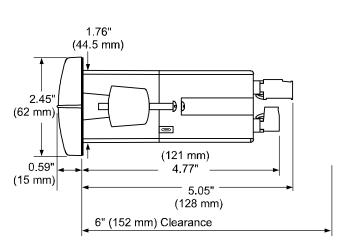
Optional Connectors Installed 4.17" (106 mm) (91.5 mm) (119 mm)
