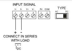
**Figure 11. DC Current Connections**
