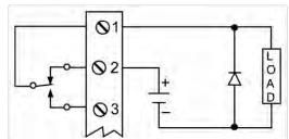
Use a diode with a reverse breakdown voltage two to three times the circuit voltage and forward current at least as large as the load current.
