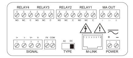
Figure 5. Connector Labeling for Fully Loaded PD6400
