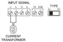
Figure 10. AC Current Transformer Connections
