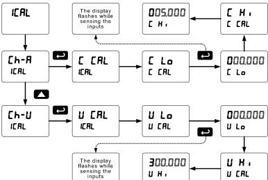
The graphic above shows the calibration of the current input. The voltage input is calibrated in a similar way.
