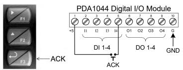
Figure 21. Acknowledge Relays w/Function Key or Digital Input
