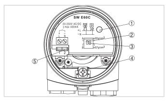
Electronics and terminal compartment, single chamber housing
